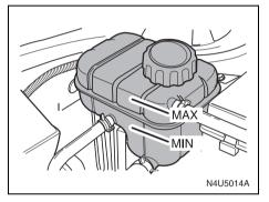
The engine coolant surge tank is located on the driver's side of the engine compartment. See "Engine Compartment Overview" in this section for more information on location.
